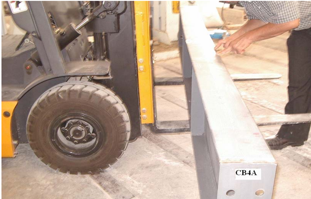
Figure 5.11: Lateral-Torsional Buckling Mode in Beam CB4A
