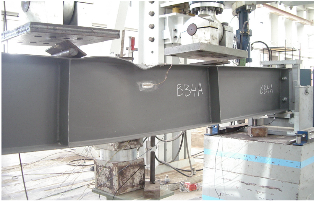
Figure 5.9: Combined Buckling Mode in Beam BB4A
