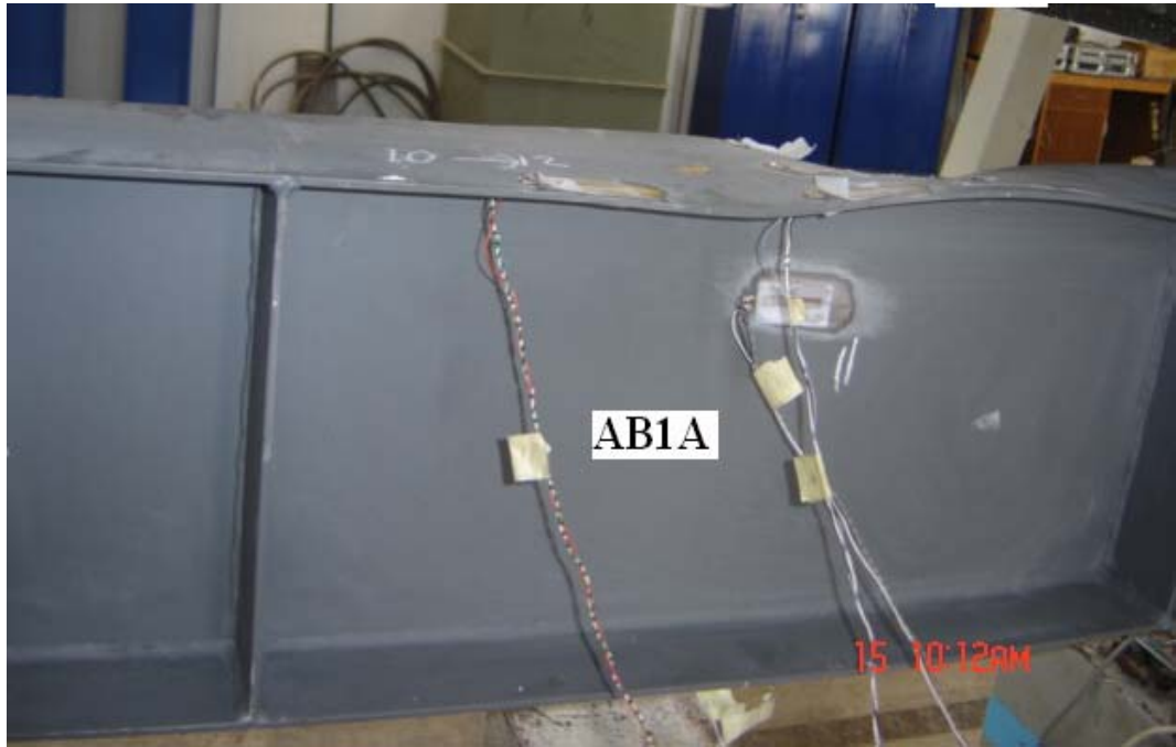
Figure 5.1: Combined Buckling Mode in Beam AB1A.
