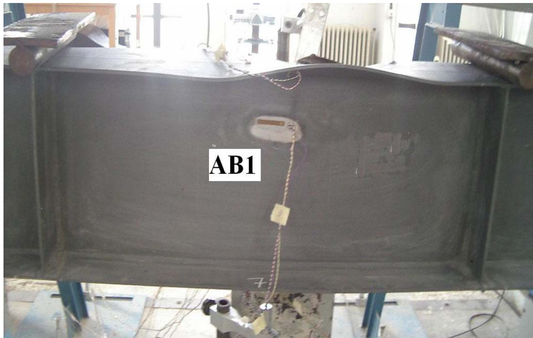
Figure 5.2: Local Buckling Mode in Beam AB1.
