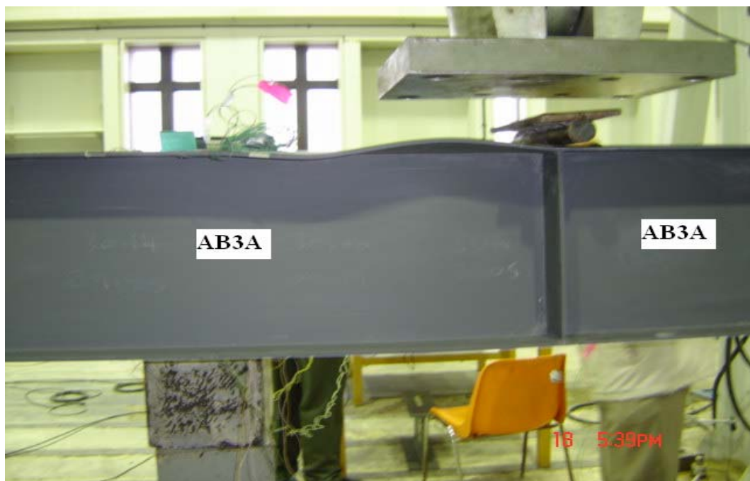
Figure 5.8: Combined Buckling Mode in Beam AB3A
