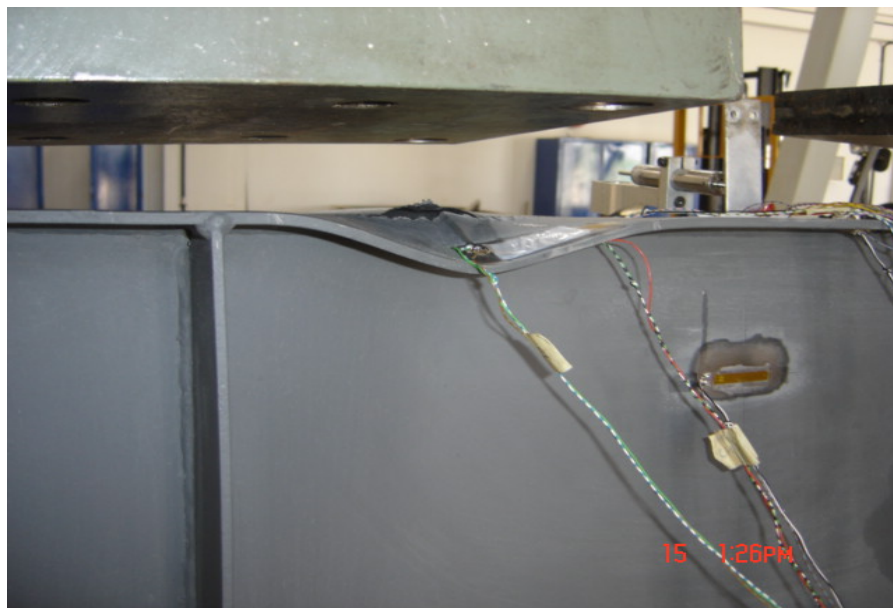
Figure 2.1: Local Buckling of I-Beam
