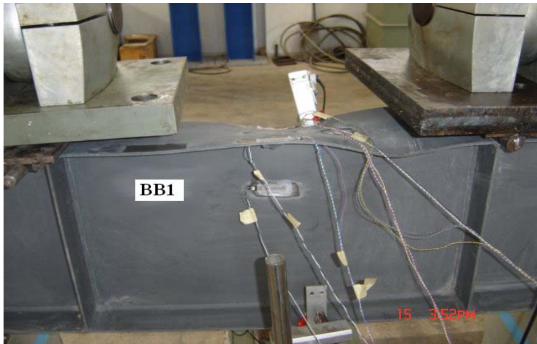
Figure 5.6: Combined Buckling Mode in Beam BB1
