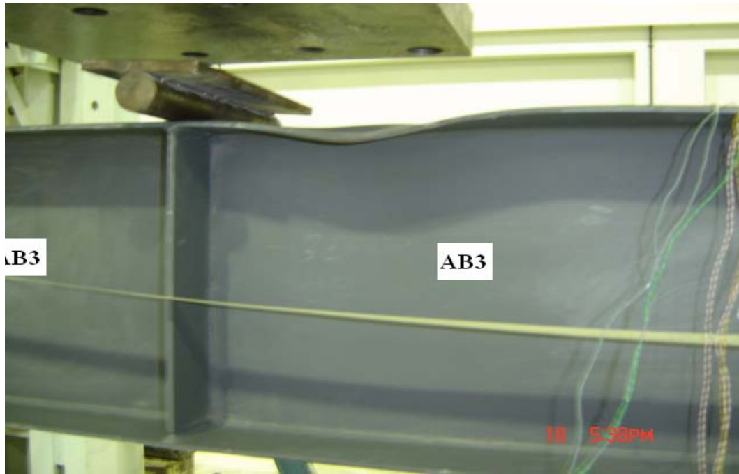
Figure 5.7: Local Buckling Mode in Beam AB3
