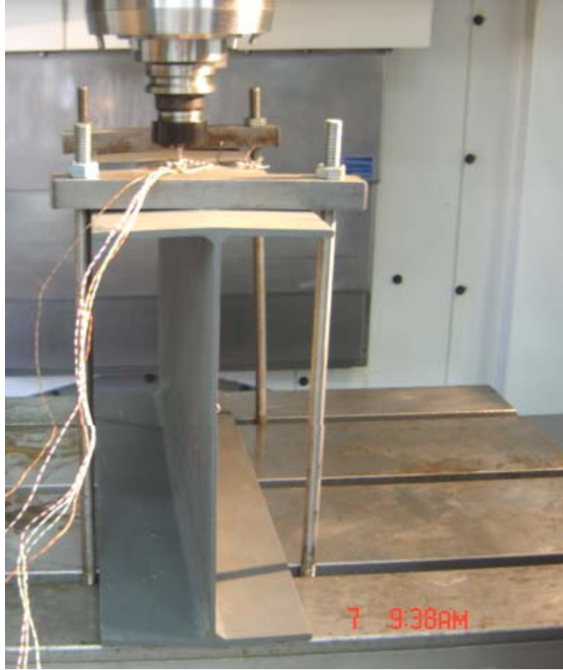
Figure 3.7: Instrumentation of Residual Stress Measurement
