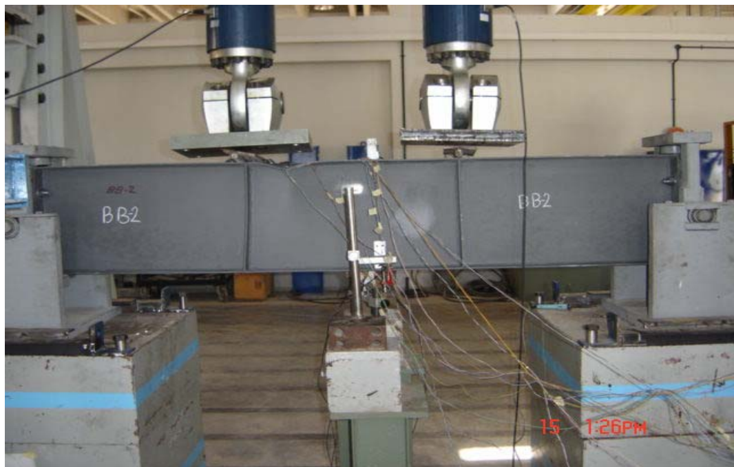
Figure 5.4: Combined Buckling Mode in Beam BB2
