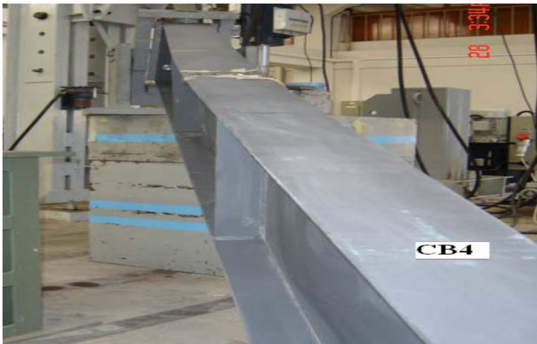
Figure 5.12: Lateral-Torsional Buckling Mode of Beam CB4
